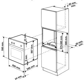
In order to ensure adequate ventilation, the back panel of the cabinet unit must be removed. Installing the oven so that it rests on two strips of wood is preferable. If the oven rests on a continuous, flat surface, there must be an aperture of at least  $45 \times 560$  mm.
